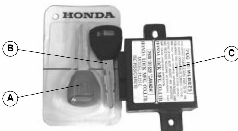
Replace the old central Immobilizer unit on the vehicle with the new one (C).
