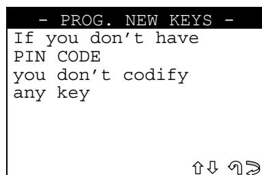
**PIN CODE:** the code comprises 6 digits and must be obtained exclusively from an authorized dealer, communicating the vehicle chassis number..
