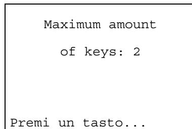
This starts programming of the keys in the vehicle, **ONLY 2 KEYS CAN BE USED**. The horn will sound for an instant.
